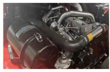
A brand new air filter with a safety filter element makes the engine air intake cleaner and more powerful.
