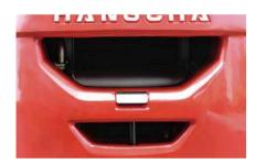
By optimizing the heat dissipation system, the counterweight heat dissipation channel is improved, the air resistance of the heat dissipater is reduced, the cooling efficiency is improved, and the reliable operation of the engine is ensured.
